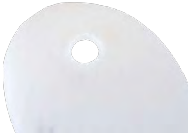
Figure 11: Plastic Accumulation With an Insulated Technovent Figura 11: ridotto accumulo di plastica con un Technovent isolato.
